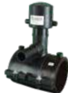
EF TAPPING TEE WITH EF END CAP EF SERVİS TE EF KEPLİ SDR11 PE100 GAS / GAZ : 10 BAR WATER / SU : 16 BAR
