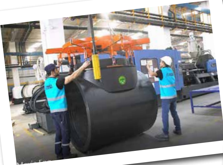
İspanya - D 1600 Çıkışlı EF Smer Testi Spain - D 1600 Outlet EF Saddle Testing
