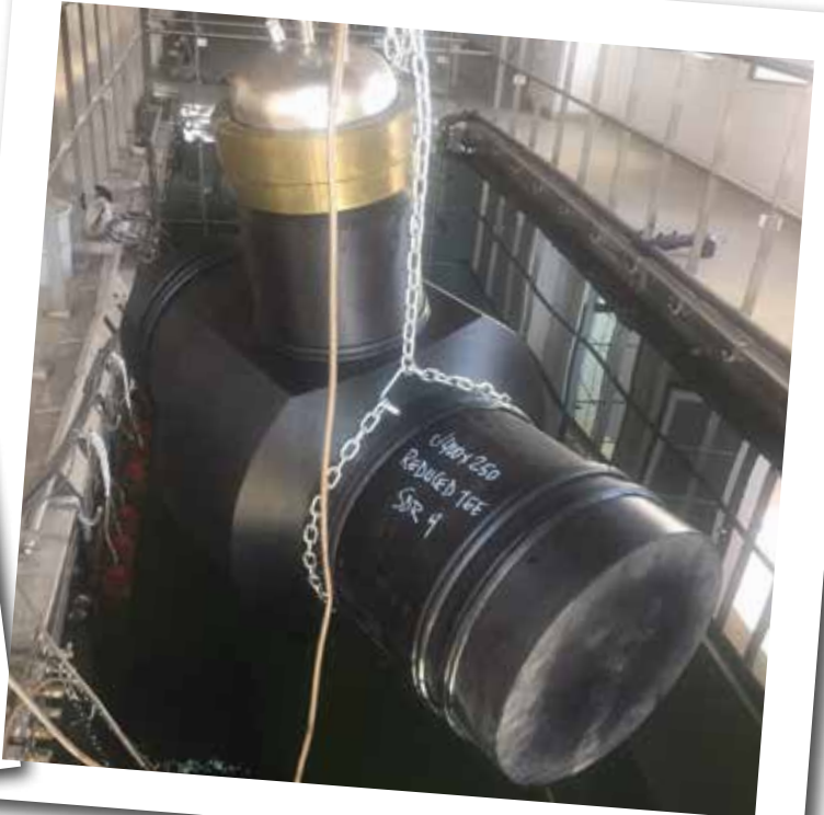
Japonya / İnegöl TE 65 Bar Testi Japan / Reduced Tee 65 Bar Testing
