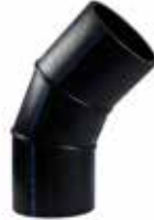
ELBOW (45°) SEGMENTED (SHORT) DİRSEK (45°) KONFEKSİYON (KISA) SDR17 PE100 GAS/GAZ : 6 BAR WATER/SU : 10 BAR TYPE/TİP : SPIGOT
