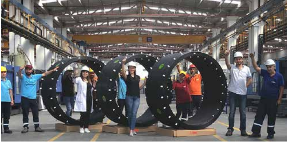
Abu Dabi - D 1600 EF DOST Manşon Abu Dabi - D 1600 EF DOST Coupler
